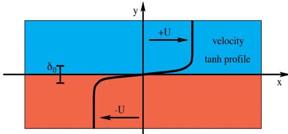
**Figure 2** Initial configuration for the mixing layer.
