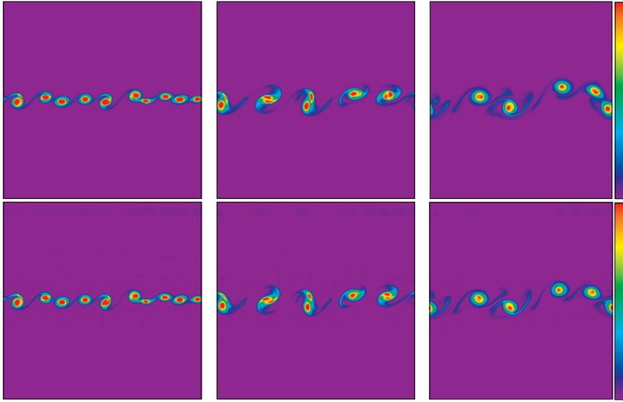
**Figure 4**  $|\omega|$  at  $t = 12.5, 25, 37.5$ . Top: spectral (vorticity-based). Bottom: method I ( $\epsilon_0 = 1-6$ ).
