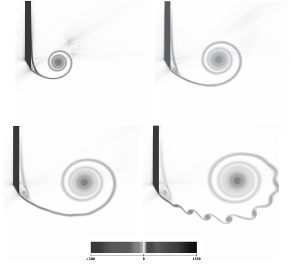
Figure 6: Flow past an impulsively started plate with a sharp wedge of angle \alpha = 30^\circ at Re = 9500 . Vorticity fields at t = 0.39, 0.75, 1.11 and 1.47 .
