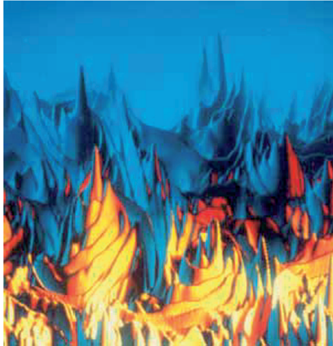
Fig. 1. Vorticity field computed by direct numerical simulation of a two-dimensional turbulent flow using a pseudo-spectral method [39]
