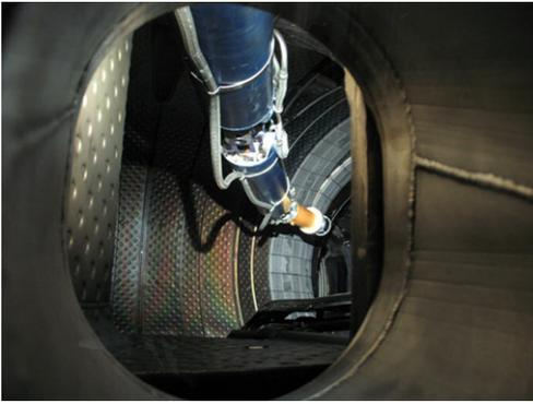
**Figure 3.** The AIA inside Tore Supra, during an inspection in ultra-vacuum and at 120 °C.
