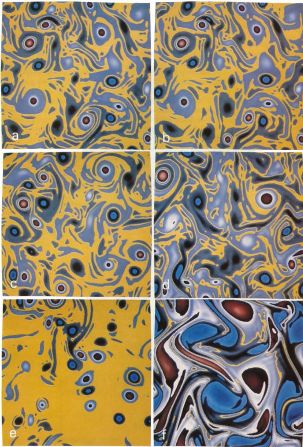
Fig. 6. Vorticity fields: "strong" components at t = 0.6 . (a) Wavelet packet: 50% strongest, (b) linear Fourier: lowest-wavenumber 50%, (c) wavelet packet: 5% strongest, (d) linear Fourier: lowest-wavenumber 5%, (e) wavelet packet: 0.5% strongest, (f) linear Fourier: lowest-wavenumber 0.5%.
