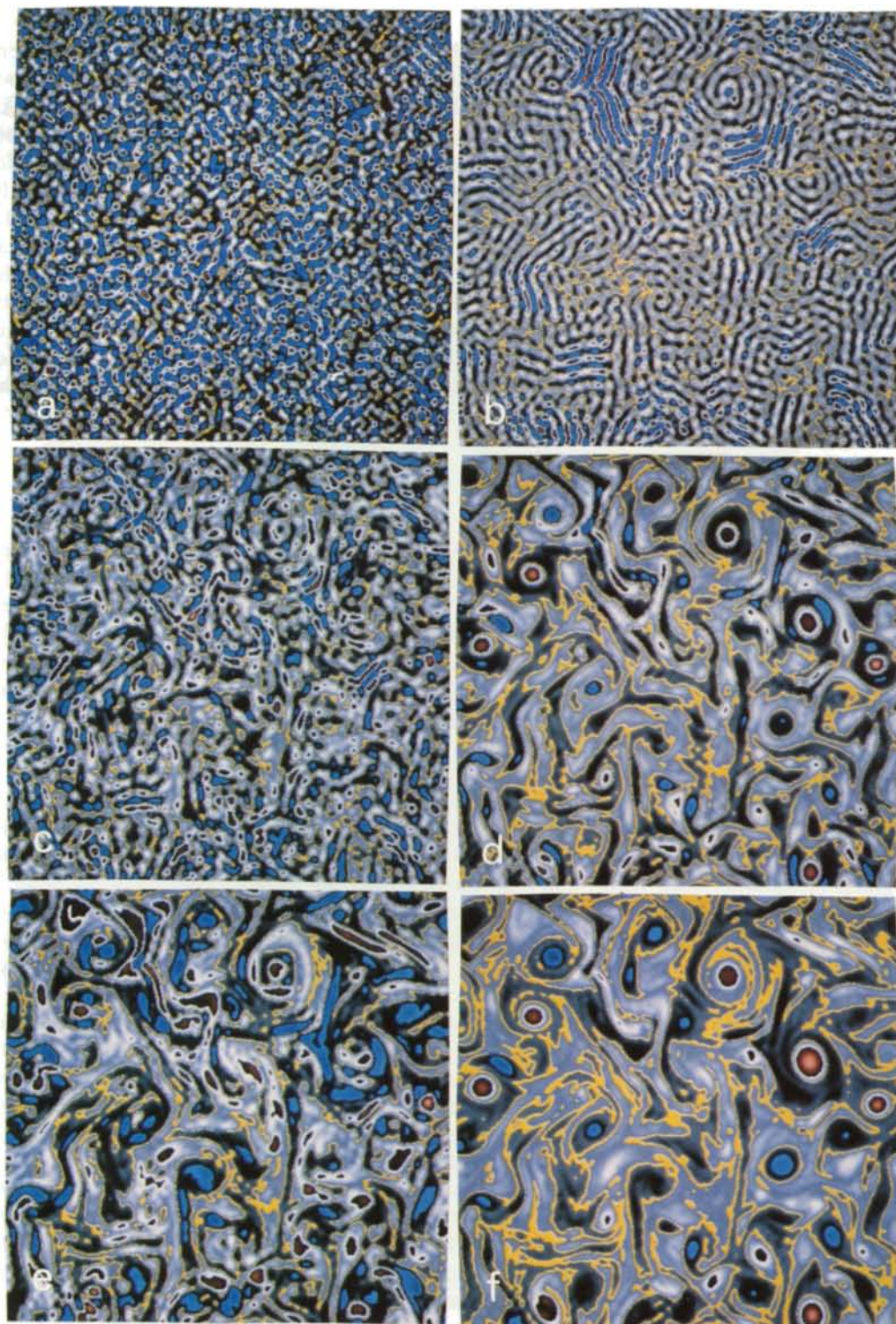
Fig. 3. Vorticity fields: “weak” components at t=0 . (a) Wavelet packet: 50% weakest, (b) linear Fourier: highest-wavenumber 50%, (c) wavelet packet: 95% weakest, (d) linear Fourier: highest-wavenumber 95%, (e) wavelet packet: 99.5% weakest, (f) linear Fourier: highest-wavenumber 99.5%.
