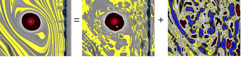
The split between coherent and incoherent vorticity can be done in this case like in the homogeneous case, but due to the penalization model, the incoherent and coherent vorticity fields leak outside of the domain. The boundary layer is captured in the coherent part. The compression achieved is approximately of a factor 10.
