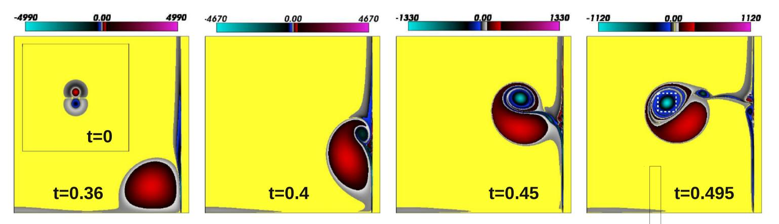
By integrating the energy dissipation rate in a region of fixed size centered on the main structure (dashed white box above), we show that we have isolated an **energy dissipating** structure.
