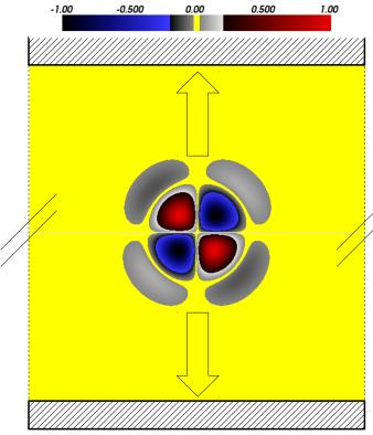
We consider a two-dimensional channel flow, with no-slip boundary conditions at the channel walls (y=0 and y=1), and periodic boundary conditions in the x direction. As initial condition, we choose a quadrupole of vorticity localized in the center of the channel, defined by the following stream function, which is designed to trigger a dipole-wall collision, as previously studied in the literature [9,12,13,17]
